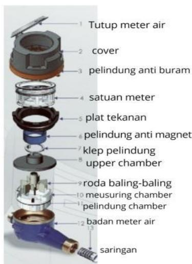
Gambar 1.1 Bagian-bagian Meter Air
