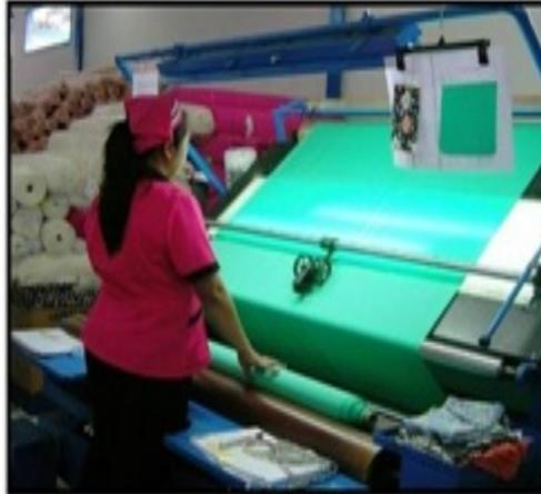
This appliance function to check the substance of before decreasing to production (whether/what destroying/perforated, or different color)
