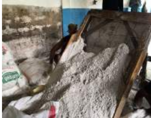
Gambar 7 Proses Pengayakan Sagu Aren
