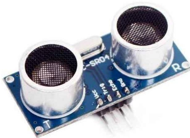
**Gambar 1.** Sensor Ultrasonik HC-SR04
