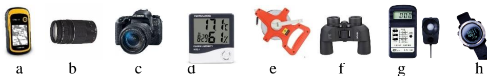
Gambar 4. Peralatan penelitian: a. GPS; b. lensa tele; c. kamera; d.thermo-higrometer; e. rol meter; f. teropong binokuler; g. lux meter; h. altimeter.
