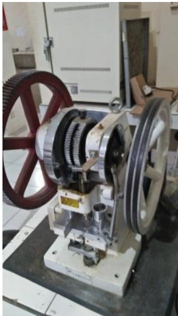
Proses pencetakan tablet ( single punch )
