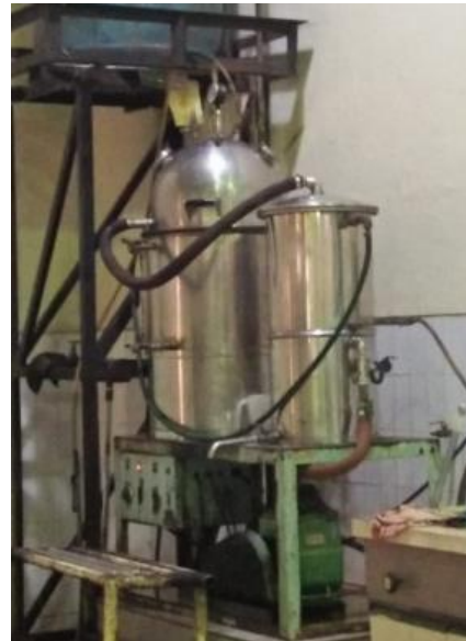
Proses pengeringan vaccum dryer
