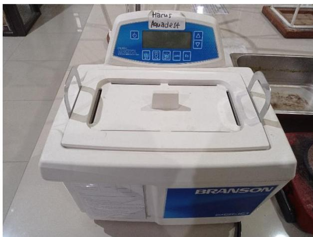
**Gambar 2.** Alat *Ultrasonic Assisted Extraction*
