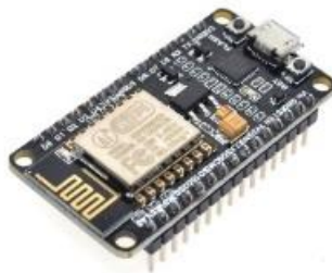
Gambar 4. NodeMCU ESP8266 (Sindhu et al., 2021)
