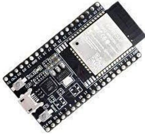
Gambar 6. Microcontroller ESP32
