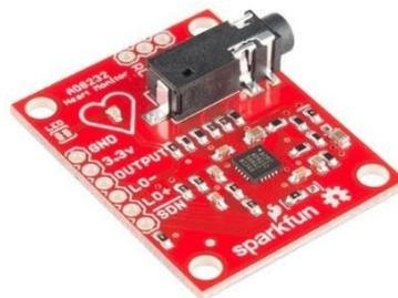
Gambar 5. Modul Sensor AD8232
