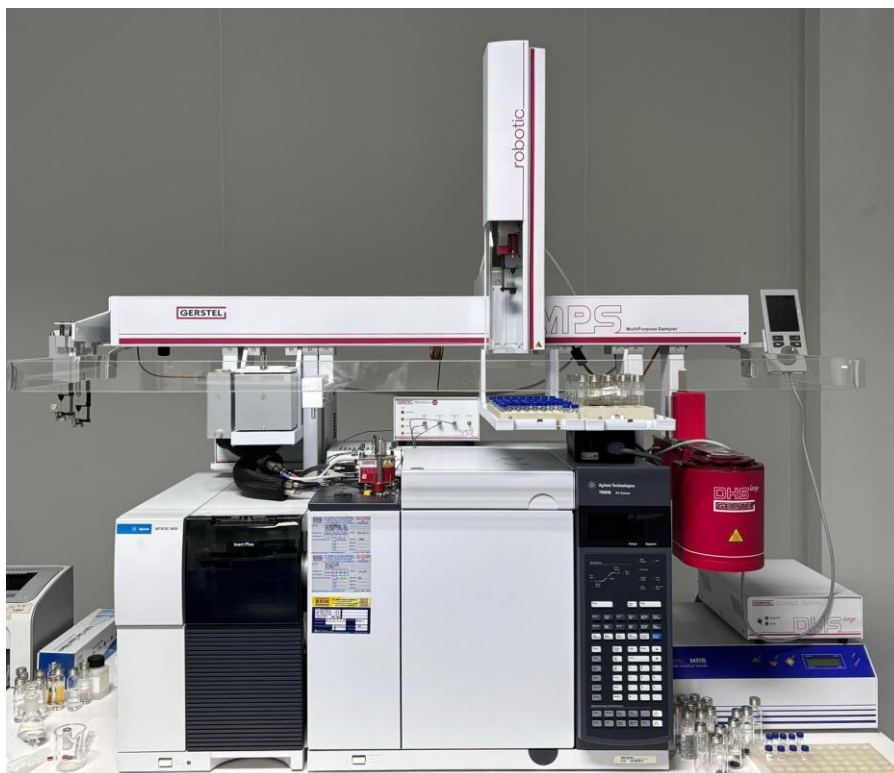
Isntrumen GC-MS Merk Agilent 7890B GC/5977B MSD With MPS Robotic by Gerstel
