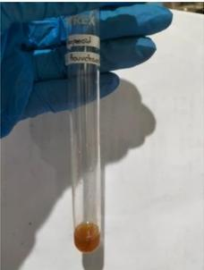
A test tube held by a blue-gloved hand, containing a clear liquid with a small amount of orange precipitate at the bottom. The test tube has a label with 'VREX' and 'Liebermann-Bouchard'. |
